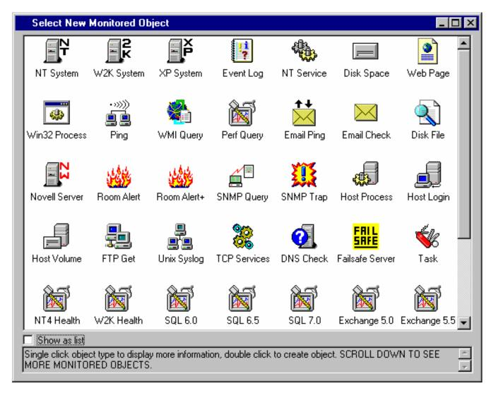
Each lcon represents a Monitored Object Type. You can single click on an lcon to get an extended description of the object displayed in the status area at the bottom of the window. Double click an lcon to create a new instance of that object. The Object specific configuration screen will then be displayed.
